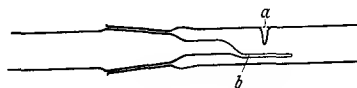
Fig. 36. Vacuum breaker, P. W. Schenk type: a ) indentation in the tube wall; b ) thin eccentric capillary tube which breaks on touching a when the ground joint is turned.
